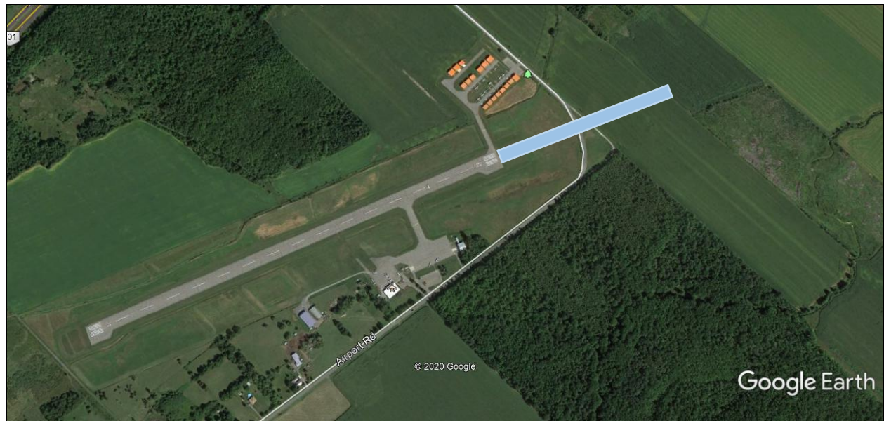
Figure 19 - Proposed Runway 10/28 expansion – 1500 feet (457m) x 100 ft (45m)
