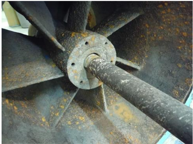
Figure 18: Pump 3 - Deep shaft wear near impeller
