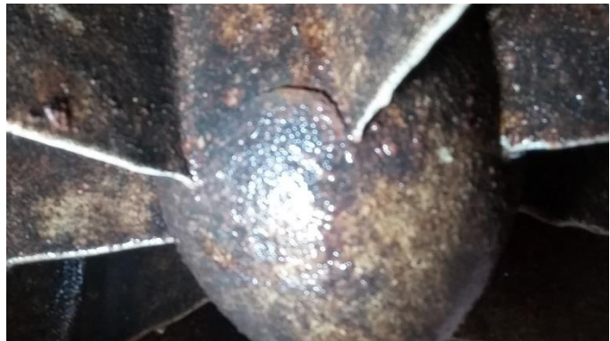
Figure 12: Pump 1 - Corroded Impeller
