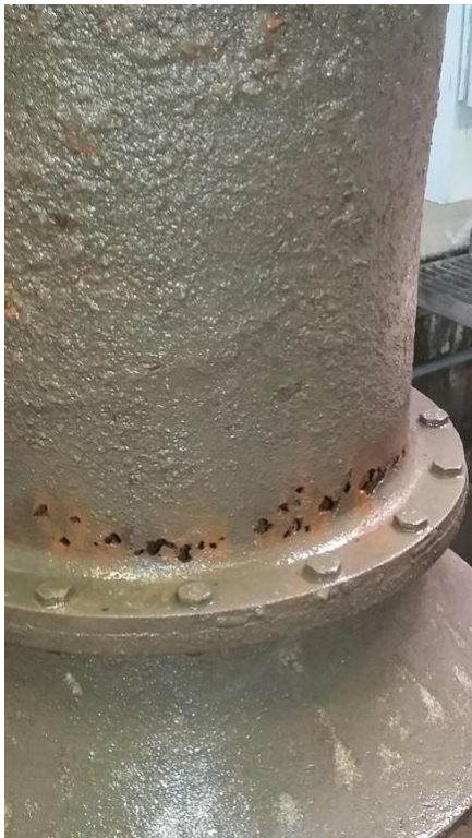
Figure 11: Pump 1 - Pitted Suction Bell
