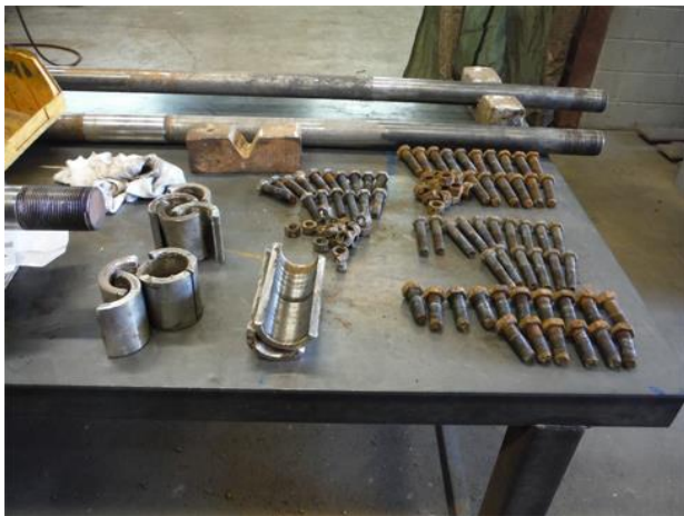
Figure 17: Pump 3 - Worn shaft couplings and bolts
