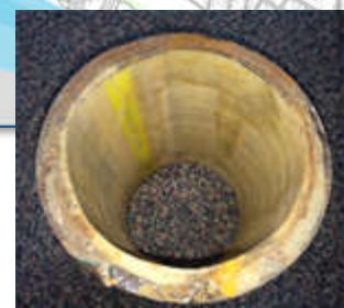
Cast Iron Watermain - After Relining
