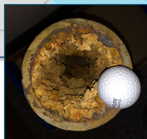
Cast Iron Watermain - Before Relining
