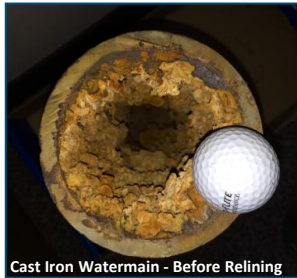
Cast Iron Watermain - Before Relining
