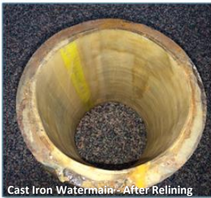
Cast Iron Watermain - After Relining
