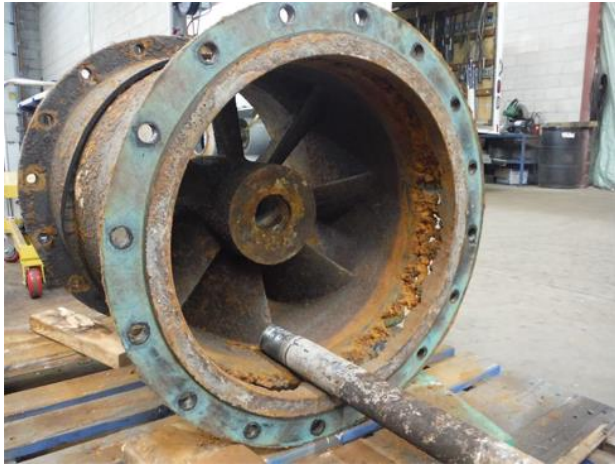
Figure 15: Pump 3 – Worn shaft sleeve
