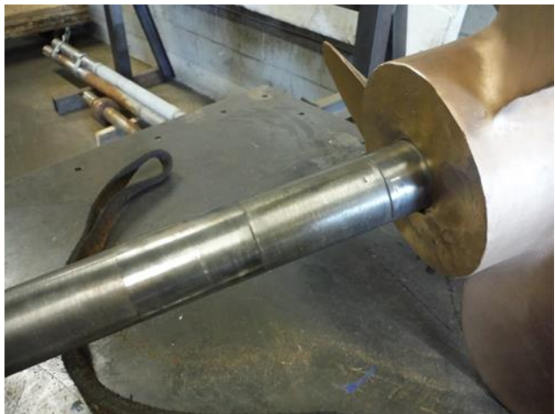
Figure 18: Pump 3 - Deep shaft wear near impeller
